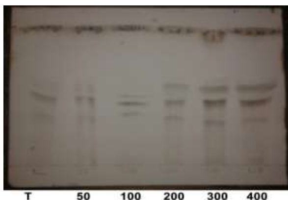
Figure 25: Photograph of the picture plate of the plate with UV 254 nm before revelation with CuSO 4 II, showing the migration of various phospholipids. (Photo of Oluwagbemiga Amos S., 2015)
