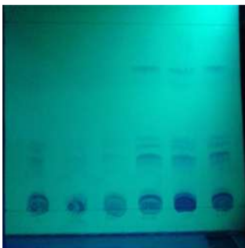
Figure 22: Picture of the plate with UV 254 nm before revelation with CuSO 4 II, showing the migration of different neutral lipids. (Photo of Oluwagbemiga Amos S., 2015)
