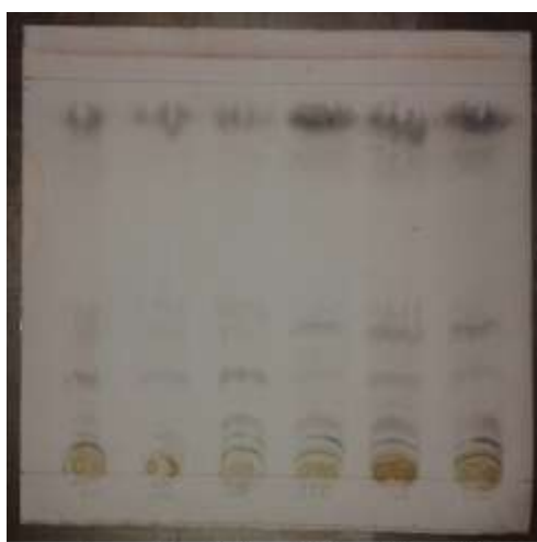
Figure 23: Photo of the plate after development with CuSO 4 II, showing the migration of different neutral lipids. (Photo of Oluwagbemiga Amos S., 2015)
