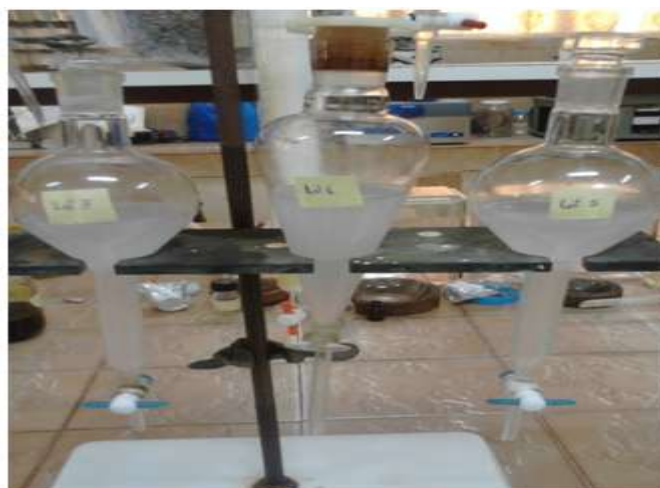
Figure 17: Phase separation photos (below) containing chloroform lipids by settling.
