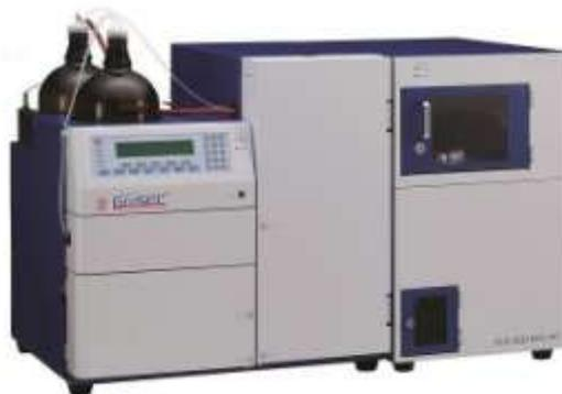
Figure 2: Instrument of gel permeation chromatography
