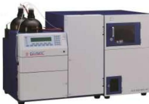
Figure 2: Instrument of gel permeation chromatography
