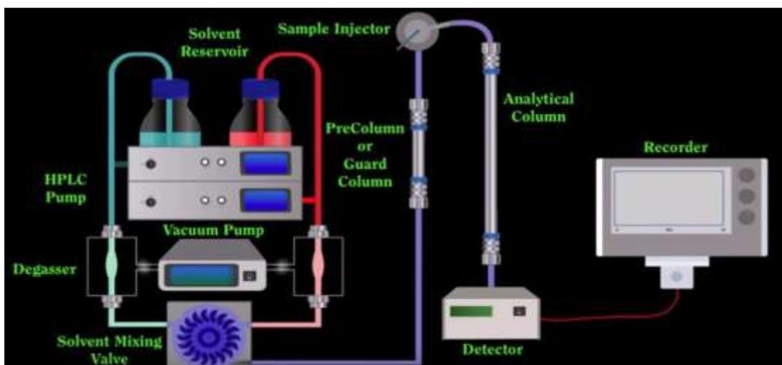
Simple working process for HPLC <sup>[54]</sup>
