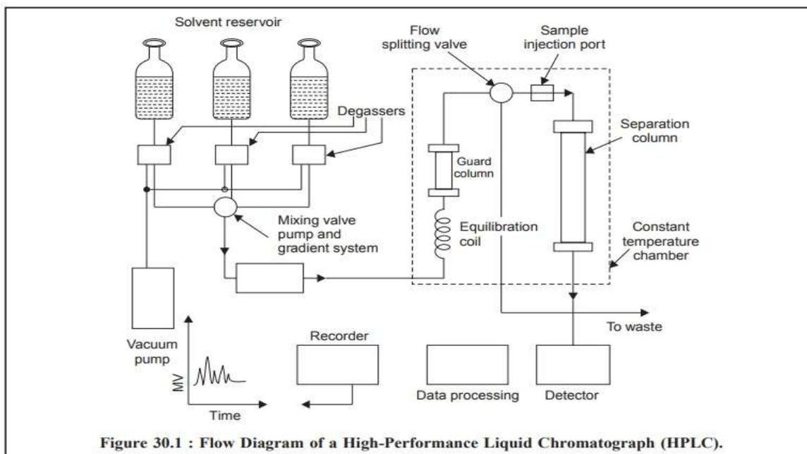
This schematic diagram shows the basic instrument for HPLC <sup>[51]</sup>
