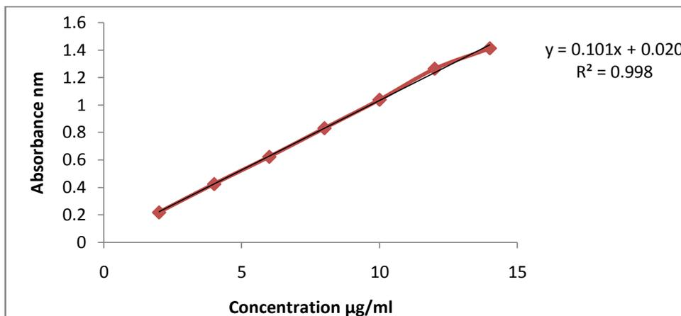
**Figure 03: Calibration graph of Levamisole HCl at 216 nm**
