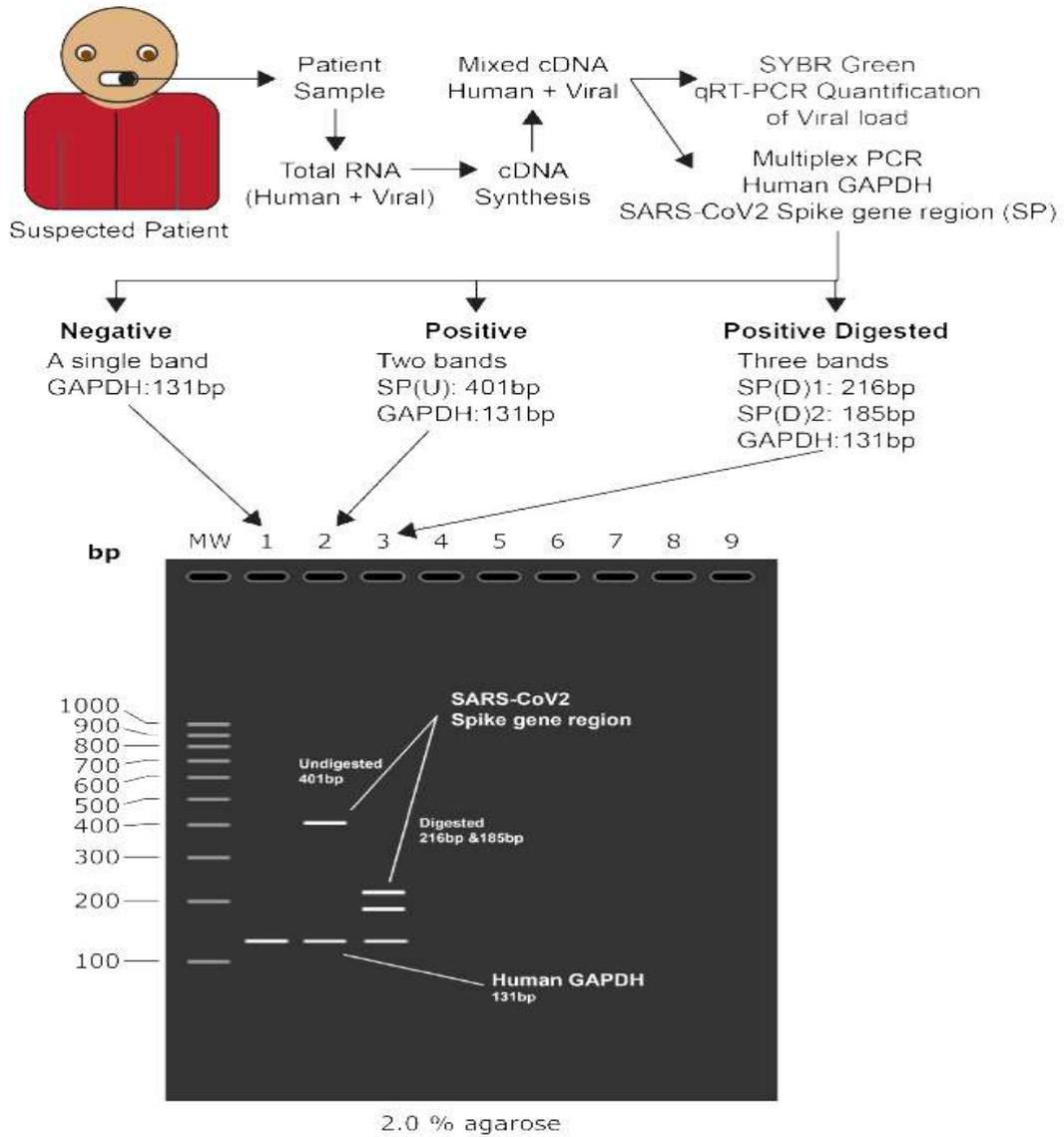
**Figure 2:** Simulated 2.0% agarose gel electrophoresis, MW: 100bp ladder; Lane 1 : Digested PCR amplicon from virus negative sample; Lane 2 : Undigested PCR amplicon; Lane 3 : Swal digested PCR amplicon.
