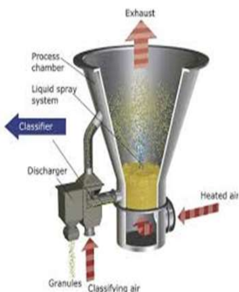
Fig 6 Fluidized bed (Air suspension system):
