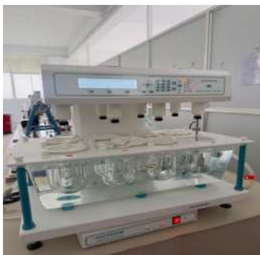
Multiple dissolution apparatus
