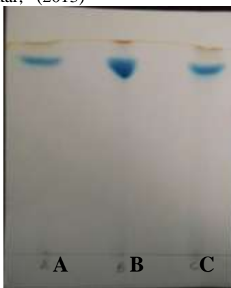
Fig.1. Thin layer chromatography of Pigment; A- Pigment from SSH-3, B- Standard pyocyanin (Sigma aldrich) and C- Pigment from HSS-6
