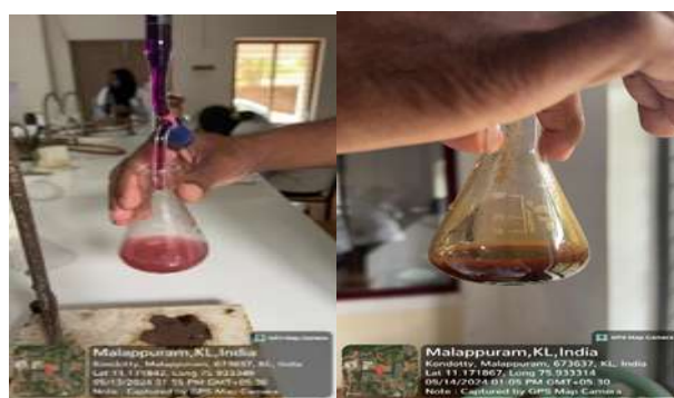
Fig 3: Titration with 0.9494 N KMnO4
