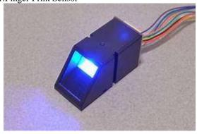
Fingerprint module is a such type of sensor in that it captures the image of the finger, and it stores the templates.
