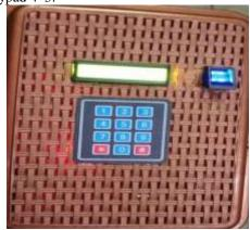
This component allows the user to enter PIN code to access the locker. Here we use 4\*3 Keypad.
