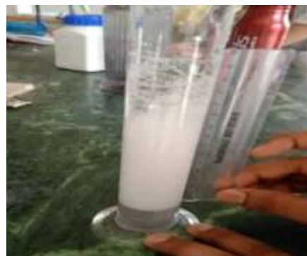
Fig. 9 Foam Height Test
