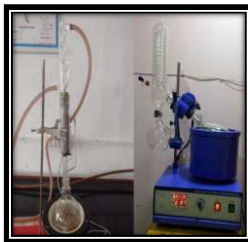
Fig.6.4 -Soxhlet apparatus & Rotary vacuum evaporator
