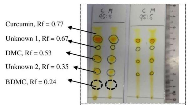
$\textbf{RF(RETENTION FACTOR)} = \frac{ \text{DISTANCE TRAVEELD BYSOLUTE} }{ \text{DISTANCE TRAVELLED BY SOLVENT} }$
