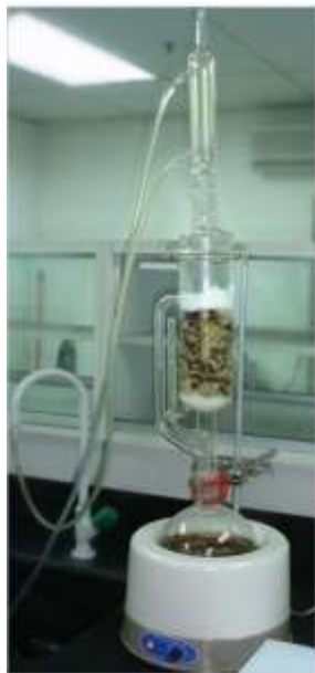
Fig: Soxhlet apparatus for plant extraction
