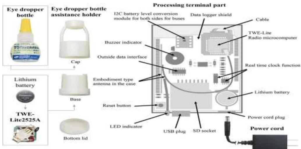
Fig 3: The Eye Dropper Bottle Sensor designed by Kazuaki Nishimura et al<sup>14</sup>
