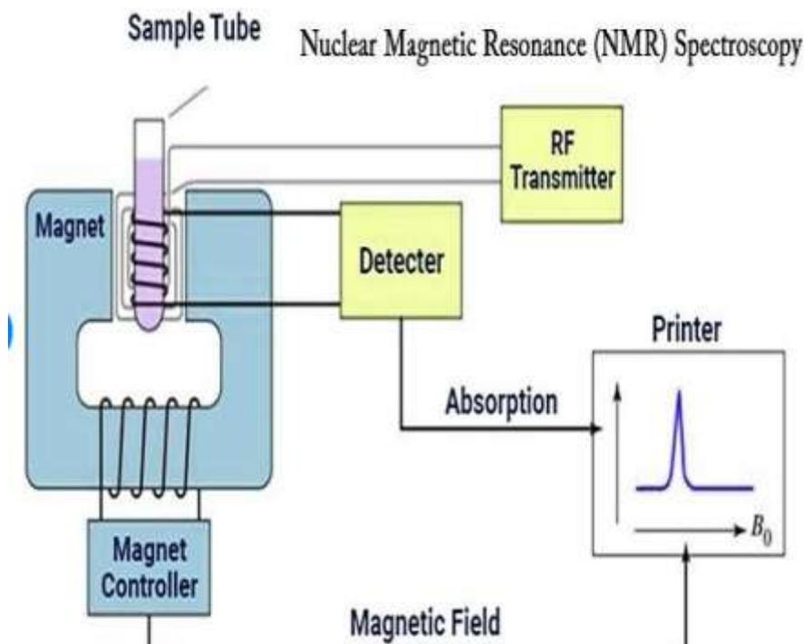
Figure 8 instrumentation of NMR spectroscopy
