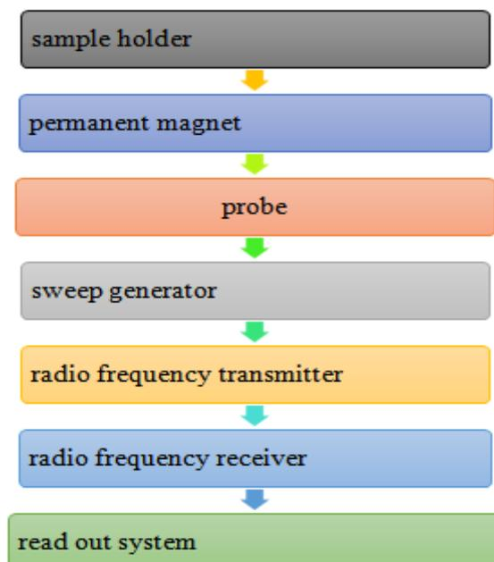
**1. Sample holder:** sample must be held in a sample holder which should be chemically inert, durable and transparent to radio frequency radiation. generally, glass tube is employed which are sturdy, practical and cheap. They are generally about 8.5 cm long and approximately 0.3 cm in diameter.
