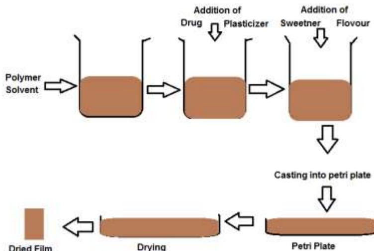
**Figure 1: Solvent Casting Method**
