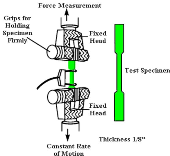
**Figure7 : Tensile Strength Measurement Device**
