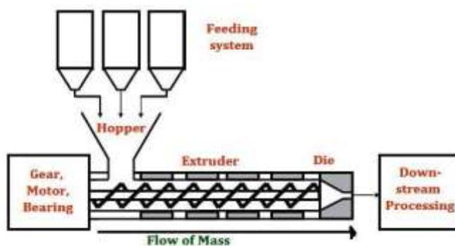
**Figure 2: Hot Melt Extrusion**
