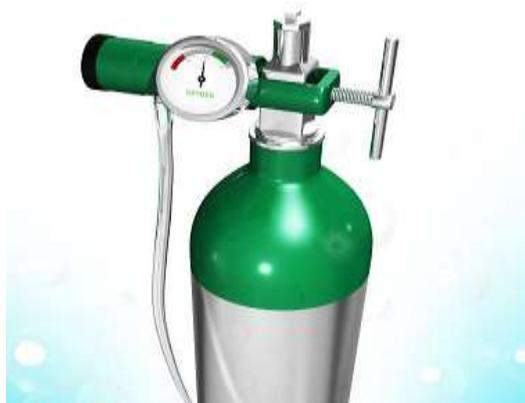
A single stage regulator is rarely used to provide constant pressure from the cylinder to the gas chromatograph. It is used in gas lines to control line pressure. However, the delivery pressure cannot be controlled as well as the dual-stage regulator. Such regulators are installed in the gas line and require constant pressure monitoring and adjustments.
