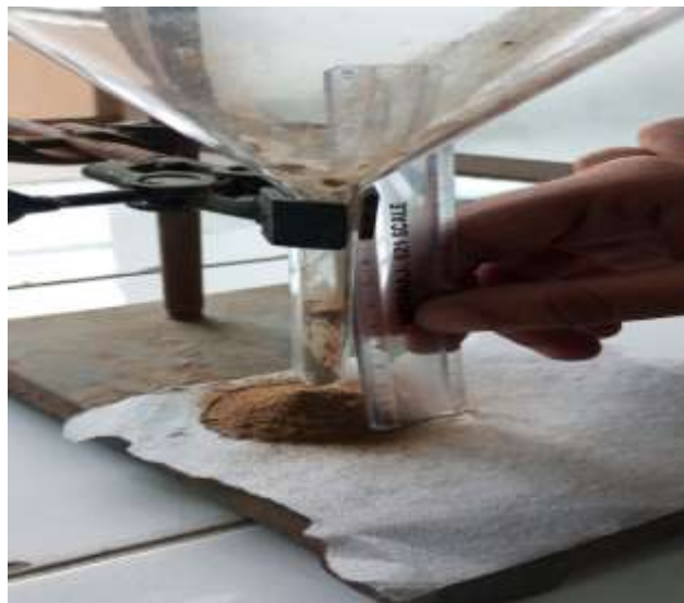
Measuring the height of the pile
