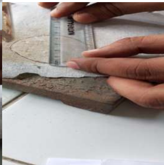
Measuring the radius of the pile
