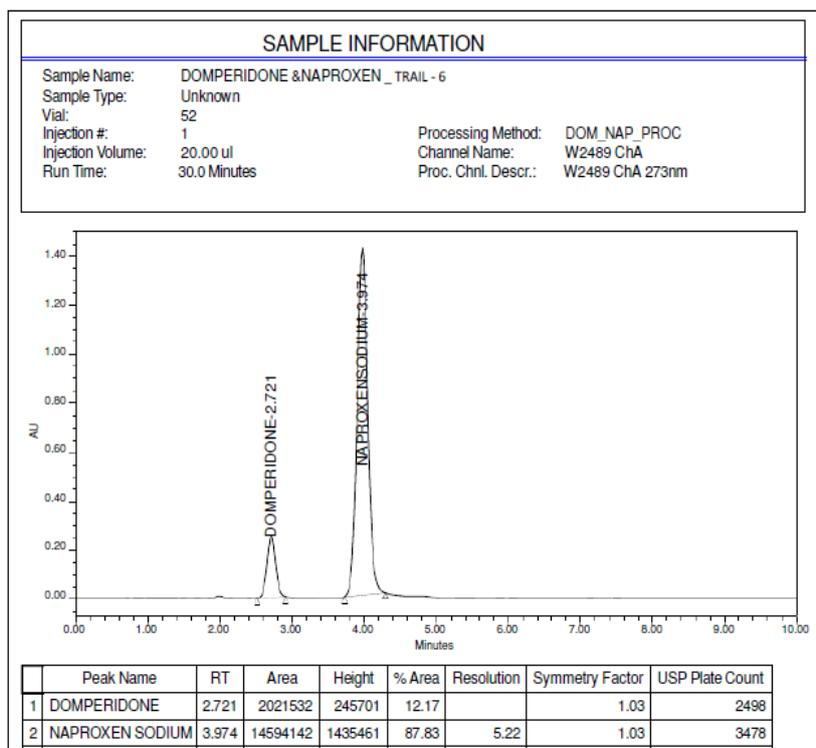
**Fig. No. 15(f): Chromatogram of Domperidone and Naproxen peaks showing good resolution with mobile phase Mix Phosphate Buffer and Acetonitrile (40:60)**
