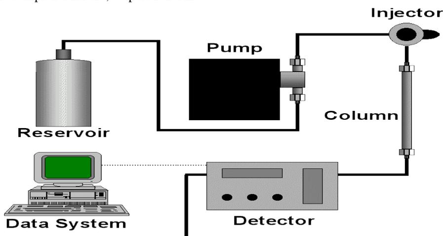
Fig.No.1: Typical Quaternary HPLC instrumentation.
