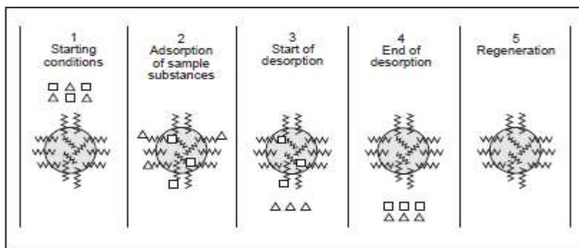
Fig. No.2: Principle of reversed phase chromatography with gradient elution
