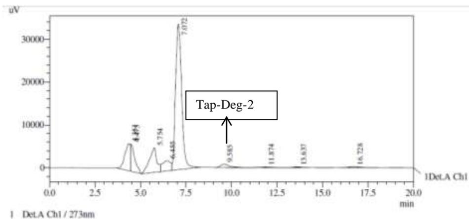
**Figure No.4 Chromatograph of TAP under alkaline hydrolysis**
