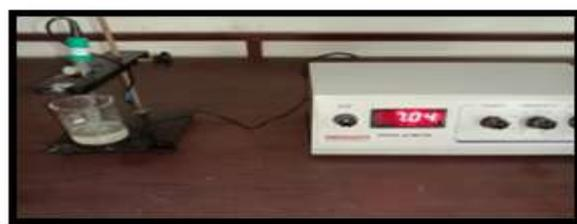
Figure 1 pH determination by digital pH meter
