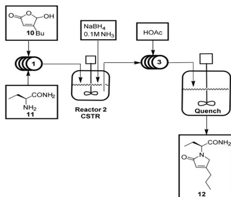
**Scheme 4.** Ongoing Flow Setup for the Reductive Amination Step in the Synthesis of Brivaracetam
