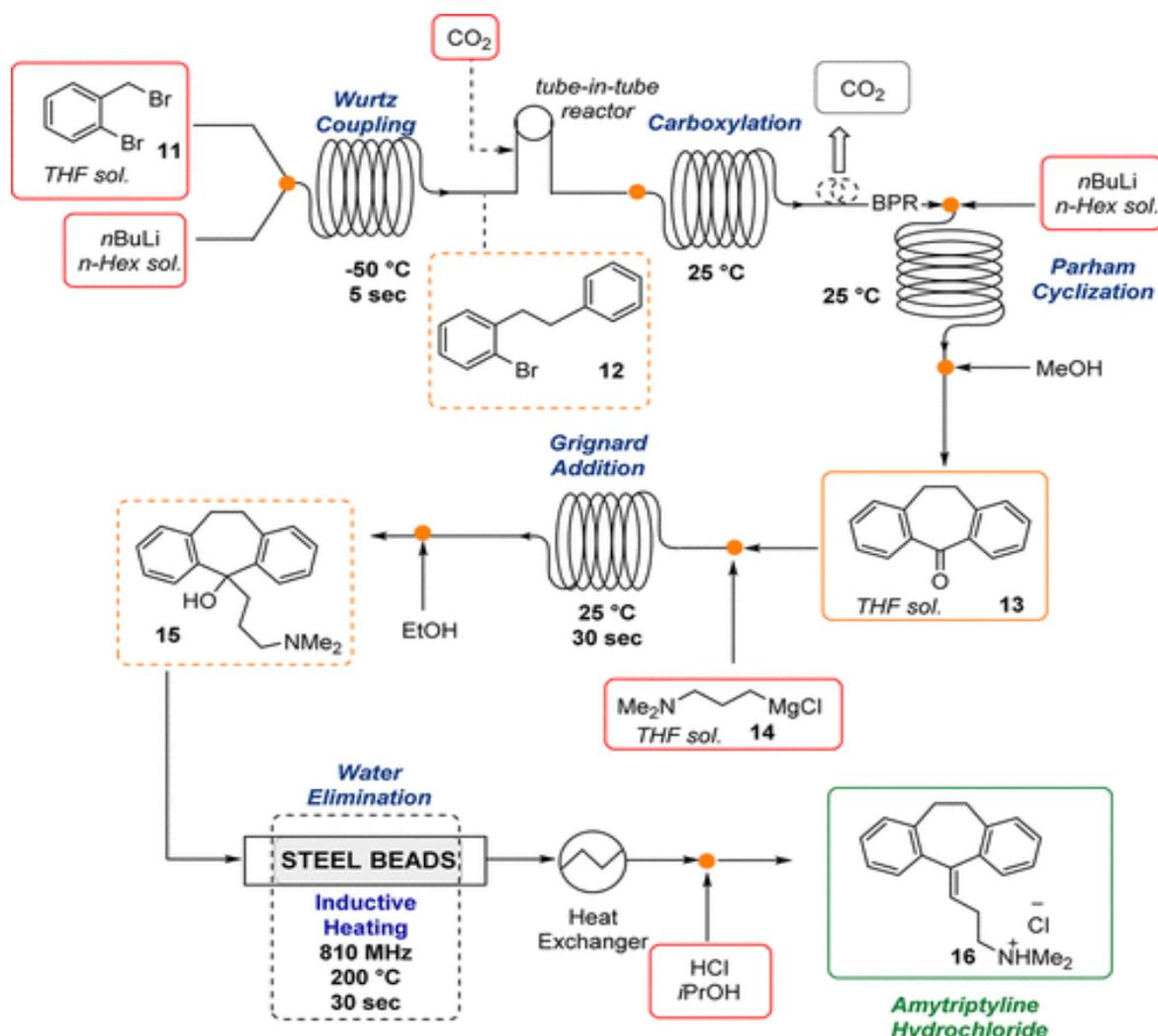
**Scheme 7.** Continuous Flow production of Amytriptyline Hydrochloride
