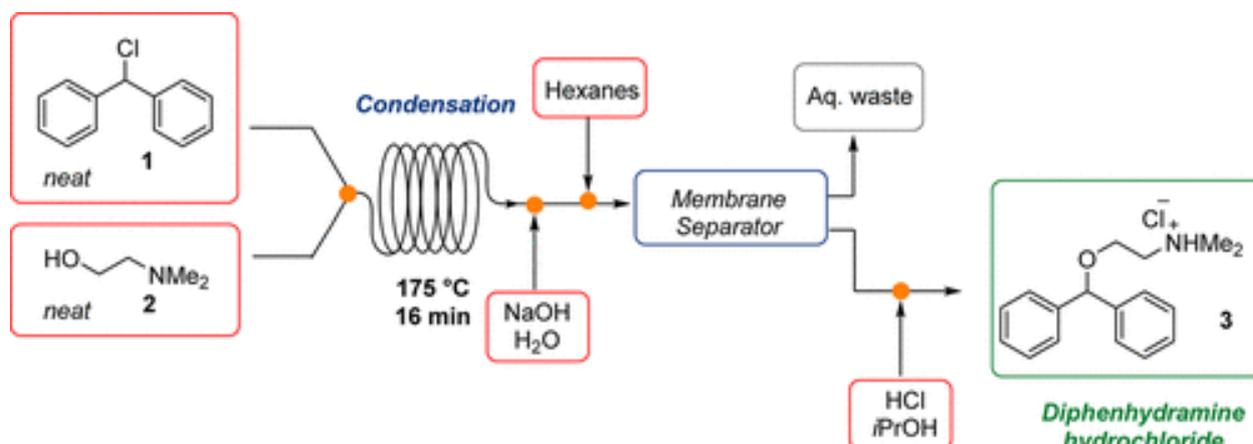
**Scheme 5.** Continuous Flow Production of Diphenhydramine Hydrochloride
