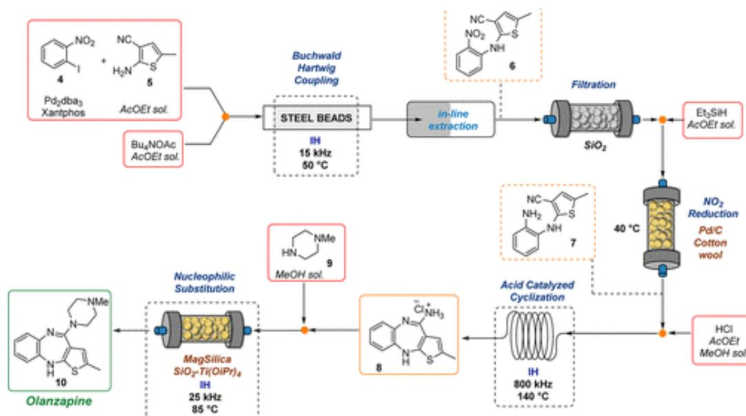
Scheme 6. Continuous Flow Production of Olanzapine
