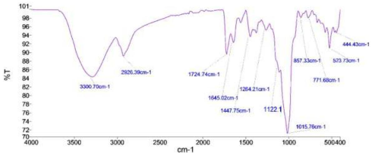
**Fig.2:** FTIR spectrum of the blank floating microspheres
