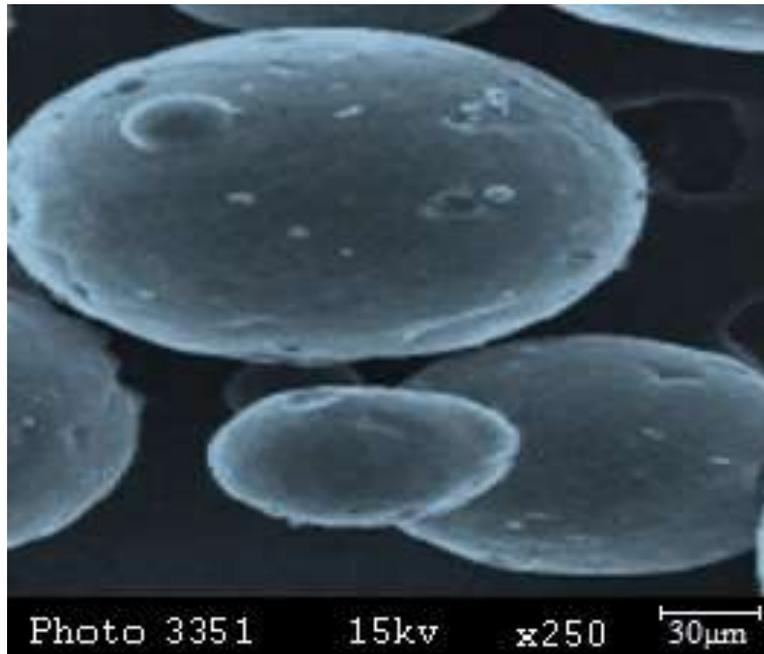
**Fig 9:** SEM photomicrograph of formulation RZS1
