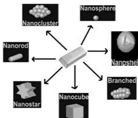
Figure 1: Various shapes of gold nanoparticles [2]
