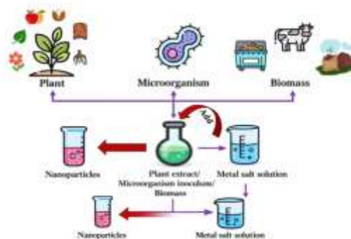
Figure 1. Schematic representation of the green synthesis of nanoparticles
