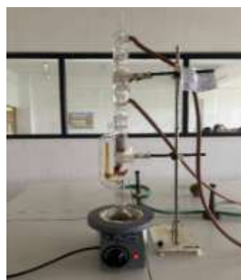
Soxhlet extraction of bark
