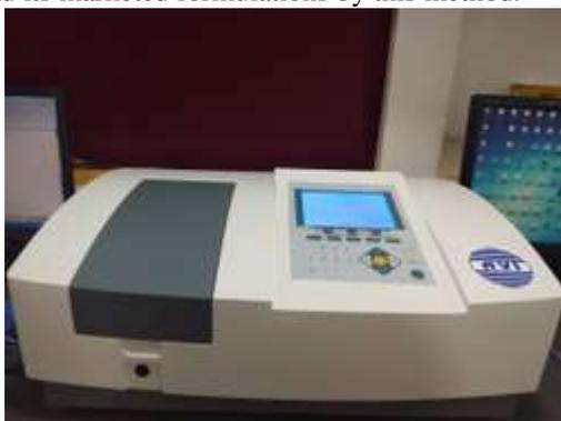
Figure 1 : Double beam UV Visible spectrophotometer
