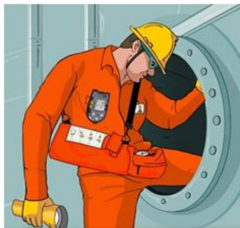
Figure 1.34: PPE for Confined Space
