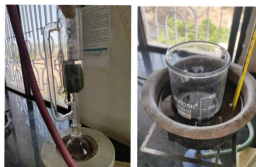
Fig. 3: Soxhlet Extraction and Evaporation of Piperine
