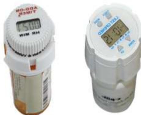
Figure 5: Left: TimerX, shows time remaining for next dose. Right: Shows the time at which bottle was last opened (Left: https://images-na.ssl-images-amazon.com/images/I/71S2GO8FEnL._SY550_.jpg ; Right: https://sep.yimg.com/ay/epill/e-pill-timecap-simple-pill-timer-8.png )
