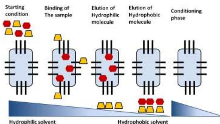
Figure.12. Steps of a reversed phase chromatography separation.
