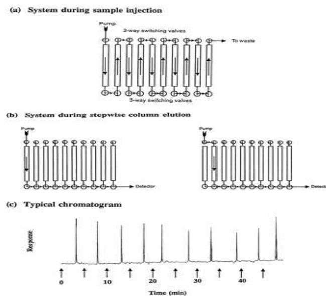
**Figure- 5 Diagram of a recycling immunoaffinity system for the determination of multiple analytes during sample application (a) and stepwise analyte elution (b) from each column in the system; and chromatogram (c) showing results obtained for the analysis of a calibration mixture.**
