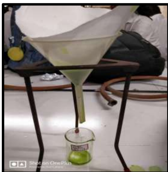
Fig 5a&5b: Filtration of the suspension using Whatmann filter paper no. 1.
