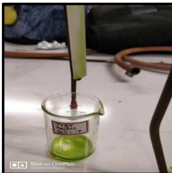
Fig 5a&5b: Filtration of the suspension using Whatmann filter paper no. 1.
