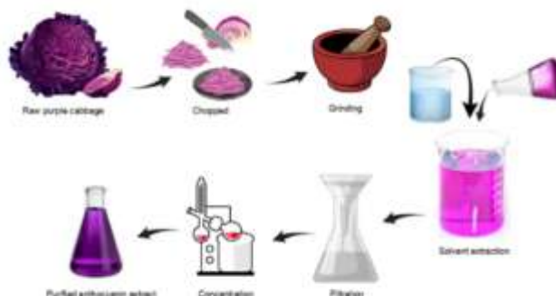
Figure. 3: Extraction of anthocyanin from purple cabbage
